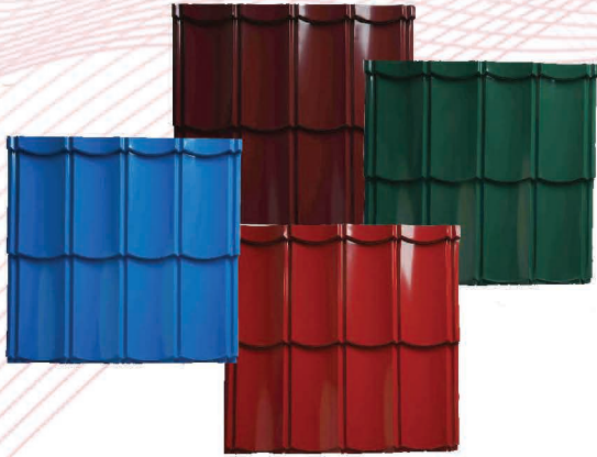
Genteng Metal Warna 2*4 (77x80 cm) Jarak Reng : 38.5 cm Tebal : 0.25 - 0.40 mm
